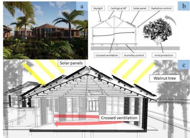
Figure 16. (a) Volumetric section view (b) Detail of bioclimatic strategies (c) Cut of proposal
