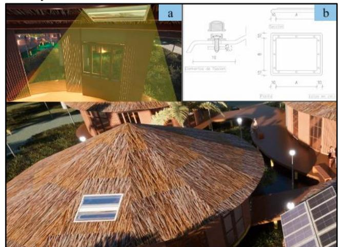
Figure 17. (a) Skylight in roofs, (b) Detail of skylight
