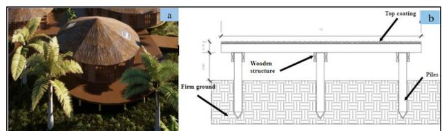
Figure 12. (a) timber piles, (b) detail of piles.
