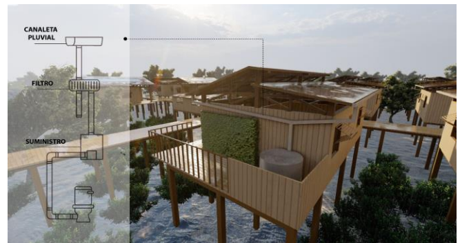
Figure 17. Gutter system with filter for rainwater purification.
