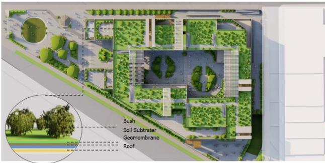
Figure 14. Green roof construction system.
