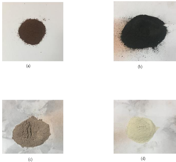
Figure 10: Collected dust samples presently used in experimental study (a) iron ore (b) coal (c) limestone (d) sandstone
