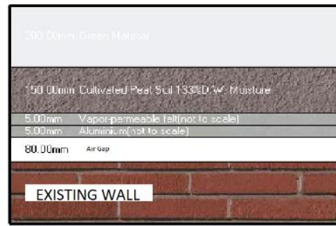
Figure 3: Green Wall Cross Section
