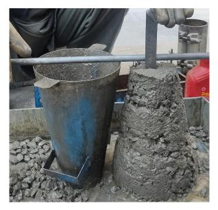
Figure 1. Measuring the value of slump of PUB.
