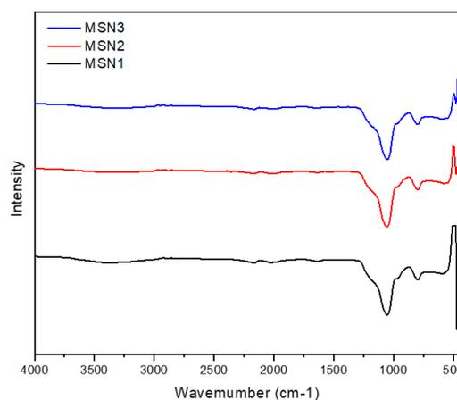
Figure 2. FT-IR spectra of the synthesized MSNs.
