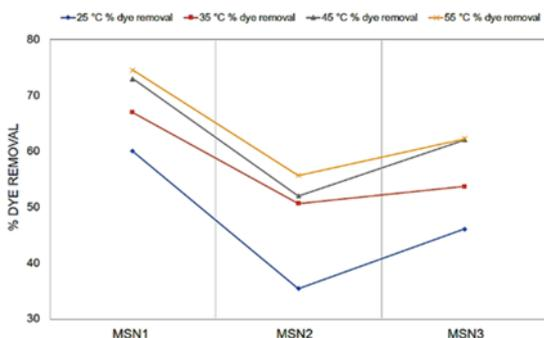
Figure 10. Effect of temperature on dye removal by MSNs
