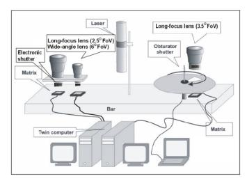
Figure 1. The Recording Unit. The objective lenses of  $3.5^{\circ}/6^{\circ}$  and  $2.5^{\circ}$  are separated from each other at the locating distance by 1 m.
