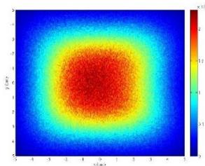
Figure 4. Spot of concentrated solar radiation obtained by simulation on the PPLR at 1.47 m from the vertex of the parabola. (The units of the color scale are W/m<sup>2</sup>).
