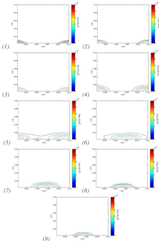
Figure 6. Distribution profiles of concentrated solar radiation on the interior walls of case 1.
