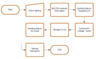
Figure 5. Flowchart of the electronic lighting monitoring system using the BH1750 sensor. Source: Author.
