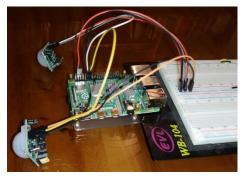
Figure 3. PIR sensors connected to Raspberry Pi 4. Source: Author.
