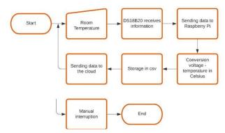
Figure 4. Flowchart of the electronic temperature monitoring system using the DS18B20 sensor. Source: Author.
