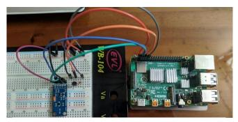
Figure 6. DB18B20 and BH1750 sensors connected to the Raspberry Pi 4. Source: Author.
