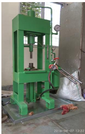
Figure 3 Actual photograph of briquetting machine
